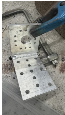
(b) Final machined and welded mount.
